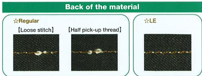
**When the thinner needle is required to avoid fabric yarn breakage (Needle hole)**
